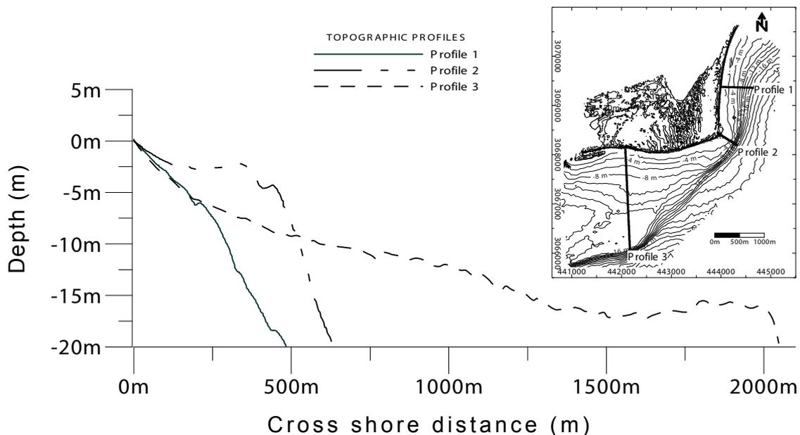
**FIGURE 4** | Topographic profiles across the insular inner shelf of Maspalomas with 90, 120, and 170°N directions to El Inglés, La Bajeta and Maspalomas profiles, respectively. Vertical exaggeration: 40.
