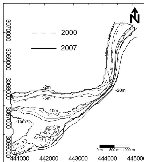
**FIGURE 9** | Landward displacement of the isobathic lines from 2000 to 2007 due to erosion of the submerged zone.
