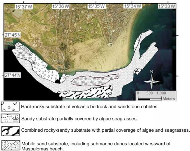
**FIGURE 5** | Cartography of the submarine sedimentary substrates in the insular inner shelf of Maspalomas.
