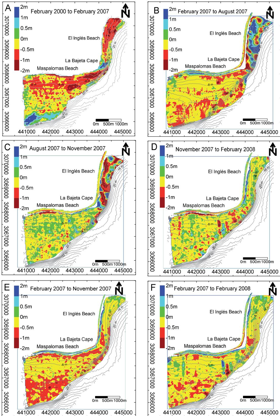
**FIGURE 8** | Sediment budget (topographic variations) A) for the submerged zone in medium-term and B-F) for the whole study area in short-term (correlative changes in B, C, and D; accumulated changes in E and F).
