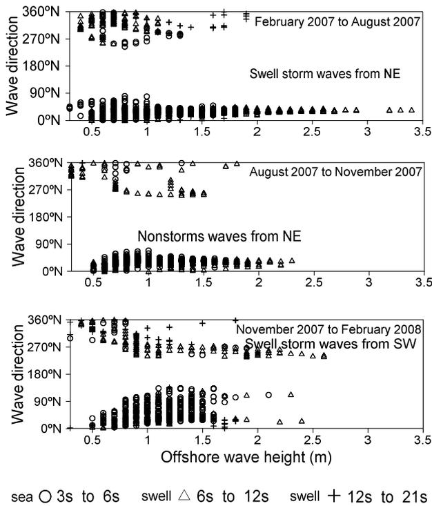
**FIGURE 10** | Offshore wave height ( $H_{s0}$ ) versus wave approach direction, after three period ( $T_p$ ) ranges and for each monitoring interval. Wave data available from Puertos del Estado.
