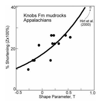
FIGURE 2 Plot of shape parameter T (T= [InF-InL]/[InL+InF]; where L, lineation is Kmax/Kint and F, foliation is  $K_{int}/K_{min}$ ) versus % shortening in pencil structures from Knobs Formation (Parés and van der Pluijm, 2003).
