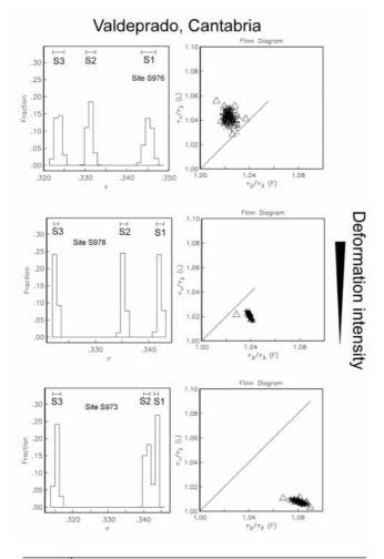
FIGURE 4 Histograms of the bootstrapped eigenvalues associated with the eigenvectors (Table 1). Each diagram includes Cartesian coordinates S1, S2, and S3 and the associated bounds containing 95% of each eigenvalue. In the corresponding Flinn-type diagrams, data from individual samples are shown as triangles, dots are average values for bootstrapped para-data sets.
