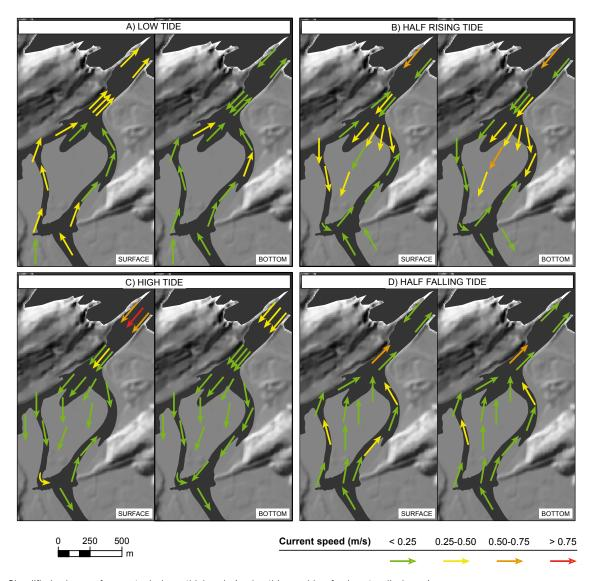
FIGURE 8. Simplified scheme of currents during a tidal cycle (spring tides and low fresh water discharge).
