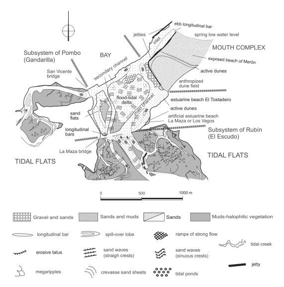
FIGURE 3. Geomorphological zonation and principal morphosedimentary and dynamic units, including the most important large scale sedimentary structures.
