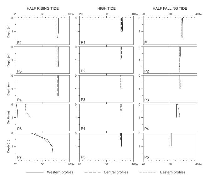
FIGURE 7. Vertical salinity records from the surface to the bottom (west, central and east) at three tide phases: half rising tide, high tide and half falling tide, for the profiles selected in the estuary.
