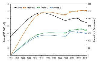
**FIGURE 4.** Evolution of Merón dune field between 1953 and 2014. The black line represents the dune field area from the jetty construction date until the most recent photograph. The gray dashed lines indicate accretion and erosion in each profile (west, center and east). The vertical dashed lines correspond to the aerial photographs used.
