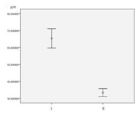
Figure 3 – Error bar (CI 95%) of the measure gap. In the chart I stands for Impregum<sup>TM</sup> whereas E stands for Express2<sup>TM</sup>.
