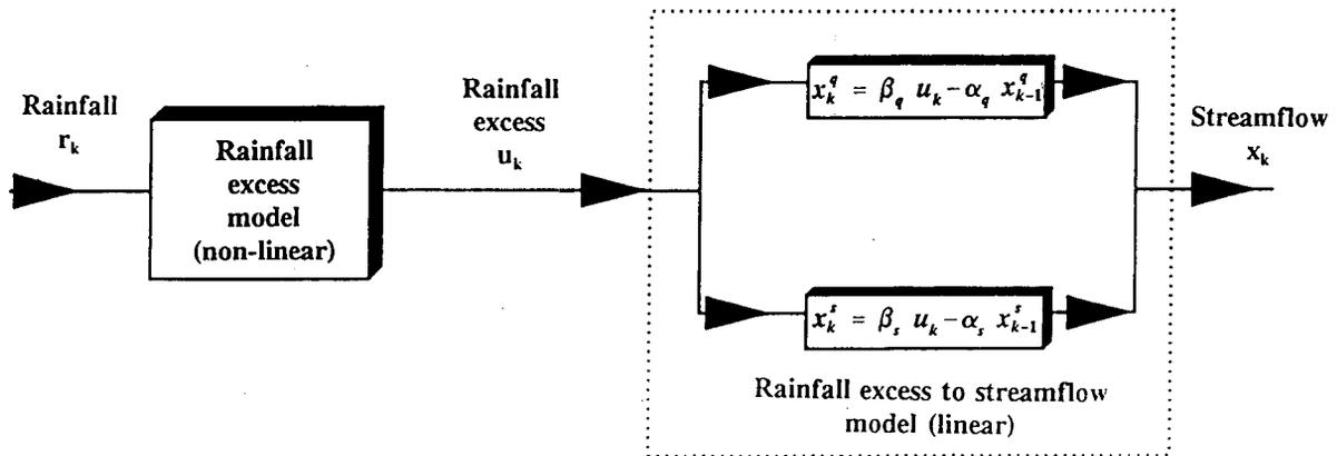
Figure 3. The IHACRES model structure using a parallel configuration of storages for quick and slow flow in the rainfall excess - streamflow module.
