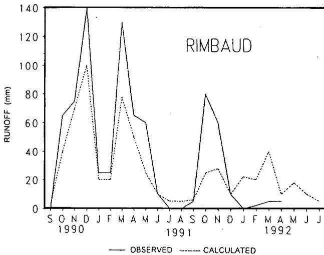
Figure 4. Monthly runoffs calculated and observed : Rimbaud catchment
