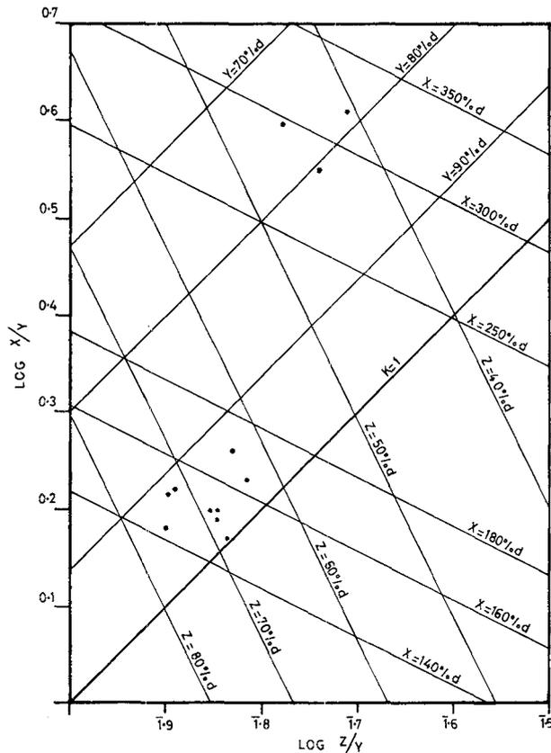
Fig. 3. Logarithmic deformation plot for mean deformation ellipsoids of the localities surveyed. ( $d$  = equivalent sphere diameter).
