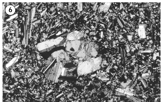
Plate 1.- Photo 1. Inequigranular porphyritic olivine basalt with microcrystalline mesostase. Phenocrysts are plagioclase (white), clinopyroxene (white-light grey with prominent exfoliation) and olivine (deep grey, affected by curved-shaped fractures, altered and frequently lacking the center of crystals (white) due to the thin-section polishing). Also note some microphenocrysts of opaque iron minerals (black) sparse in the mesostase. Scale bar is 0.32 mm. Plane parallel light (PPL). Sample 311S. Photo 2. Hypohyaline inequigranular vesicular basalt, locally with trachytic texture marked by plagioclase laths and phenocrysts (white and dirty grey, note the differential alteration following concentric growth bands of contrasting composition). Upper left is a hollow vesicle. Scale bar is 0.32 mm. Plane parallel light (PPL). Sample 318S. Photo 3. Holocrystalline inequigranular porphyritic olivine basalt with microcrystalline to intergranular mesostase. Phenocrysts as in photo 1: note in the upper centre sector an unaltered olivine phenocryst that has undergone thermal shock as shown by curved jig-saw fractures. Scale bar is 0.32 mm. Plane parallel light (PPL). Sample 307S. Photo 4. Hypohyaline inequigranular porphyritic olivine basalt with intergranular to microcrystalline mesostase. Note the presence of a triangle-shaped sector with brown (dark grey in the photo) glass with skeletal hollow sections of plagioclase that are evidence of supercooling, lying at the right of the large clinopyroxene phenocryst. Mesostase consists of medium-sized idio- to hypidiomorphic plagioclase laths
