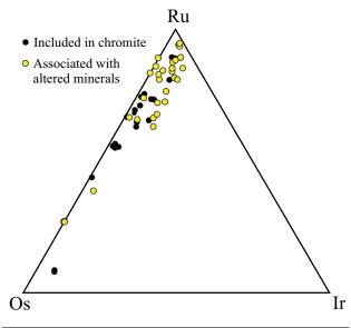
FIGURE 9 | Electron microprobe composition (Atomic %) of Platinumgroup mineral sulfides of the laurite-erlichmanite series, associated with the chromitites of Santa Elena. Both suites of PGM included in chromite or associated with altered minerals show consistent composition.
