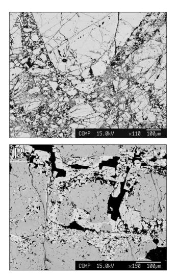
FIGURE 5 Back scattered electron images of polished sections from the Santa Elena chromitites. A) Coarse grained chromitite with strong brecciation controlled by shear planes. B) Ferrian chromite alteration (light grey) developed along cracks and fissures in massive chromitite.
