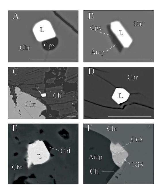
FIGURE 8 Back scattered electron images of Plainum-group minerals associated with the chromitites of Santa Elena. L: laurite ( $RuS_2$ ). White spot visible in E and F are due to an Os bearing phase, possibly native Os. Scale bar = 10µm.
