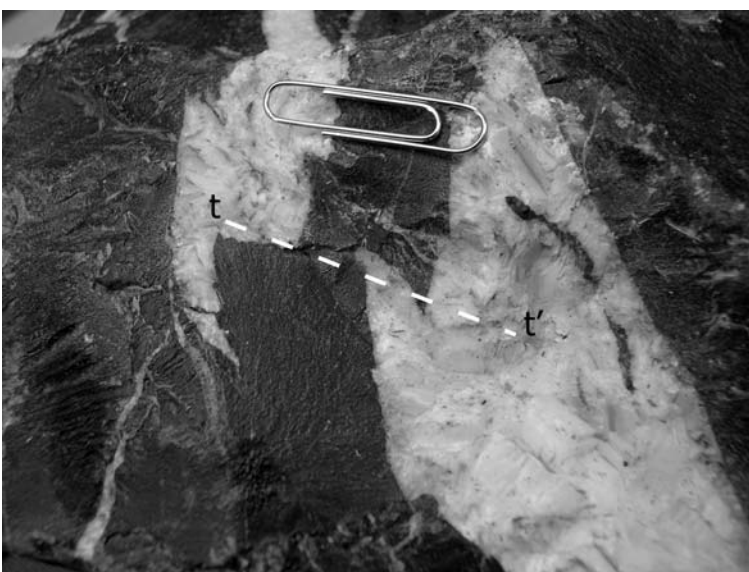
FIGURE 5 | Dolomitic breccia in the Cambrian Dunham Dolomite of NW Vermont and southern Quebec. The two black blocks of host rock at center were differentially displaced along an east-west fault t' , dashed, that starts and ends at the centers of the veins but that does not affect the walls. This means that t' is a transform fault, and requires that the observed displacement of the blocks relative to each other was forcibly driven by the white veins as they grew.
