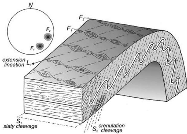
FIGURE 7 | Draft of the structural style, geometry and relationship between the cleavages, the folds and the rock fabrics in the Fuegian Andes observed in the Ushuaia area in the Yahgán and Lemaire Fms. In the upper left lower hemisphere equal area plots contours of the F1 and F2 folds hinges.
