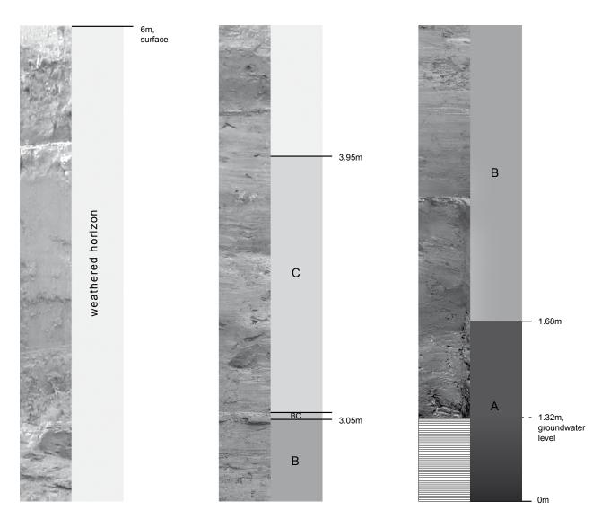
FIGURE 8. Exposed deposits of excavation site "Menat 2" illustrated as a stratigraphic column, presented here in three rows. The basalmost section was below the water level. The sequence is divided into the three intervals A, B, C (differentiated in the text) and the uppermost strongly weathered horizon.
