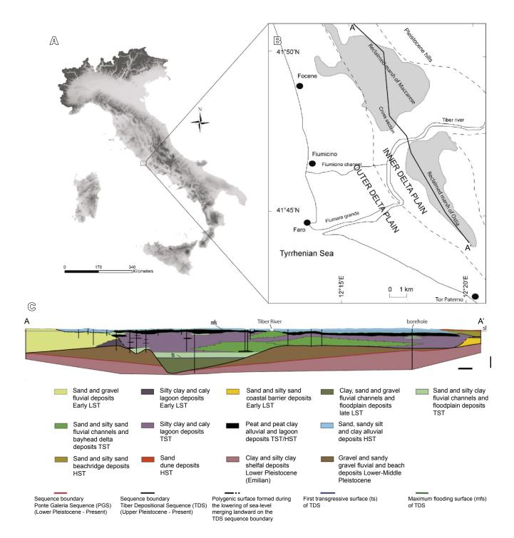
FIGURE 1. Location of the study area on 20m DEM. A); Tiber Delta domains (redraw after Bellotti et al., 2007) B); cross section of the delta plain (redrawn after Milli et al., 2013). The track of the cross section c) is shown in b). In the cross section C) the peat layers that characterize the Maccarese and Ostia ponds are shown.
