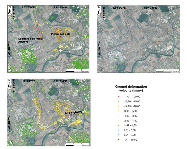
FIGURE 5. Ground deformation velocity maps in the area of Maccarese. A) ERS 1/2 (1992–2000); B) ENVISAT (2003–2005); C) RADARSAT-1 (2003–2006).
