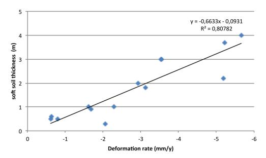
FIGURE I. Correlation diagram between PS velocity and soft soil thickness in Ostia area.
