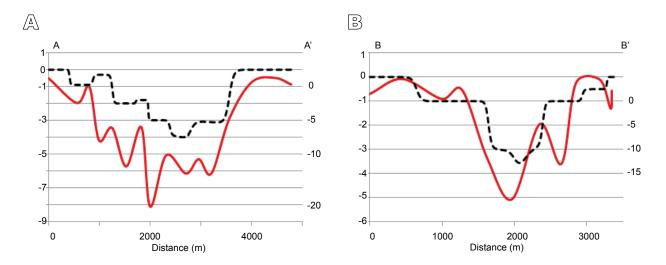
FIGURE 11. Deformation rate variation along the two geological cross-sections in the Ostia area (A–B). Left y-axe: thickness of the peat layers (in meters); right y-axe: mean PS velocity (in mm/y). The red line represents the profile based on the punctual PS file and the black dashed line represents the peaty horizon thickness.
