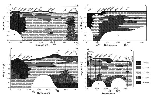
FIGURE 7. Reconstruction of the subsurface stratigraphic profiles in the Maccarese area.
