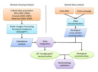
FIGURE 2. Proposed workflow to use PSInSAR data to support geological interpretation of sub-surface data analysis.
