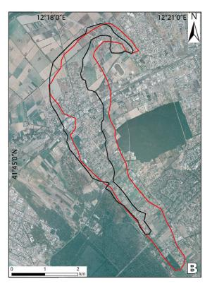
FIGURE 12. 2D reconstruction of the extension of the peat layer in A) Maccarese and B) Ostia ponds. Pond limits (black polyline) determined using PSinSAR data and boreholes; in red pond boundary from the literature (Giraudi, 2011 for Maccarese pond and Geolithologic map of Rome municipality for Ostia pond).
