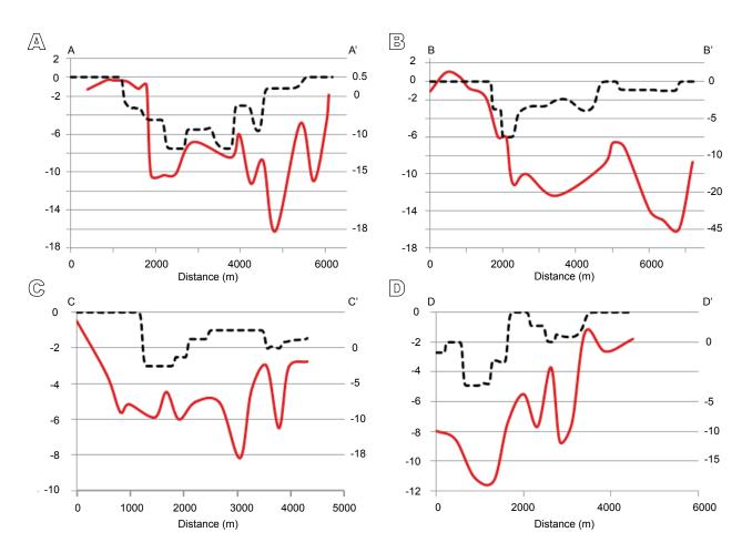
FIGURE 10. Variation of deformation rates along the four geological cross-sections in the Maccarese area (A–D). Left y-axe: thickness of the peat layers (in meters); right y-axe: mean PS velocity (in mm/y). The red line represents the profile based on the punctual PS velocity and the black dashed line represents the peaty horizon thickness.
