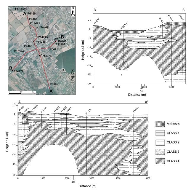
FIGURE 9. Used boreholes and geological cross-sections in the Ostia Antica area. The black dots with the identification code indicate the location of the boreholes.
