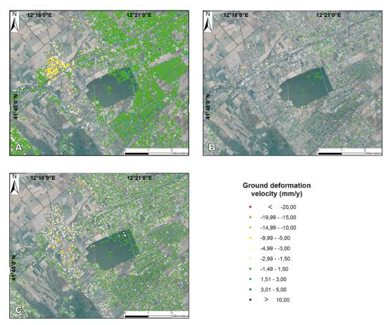
FIGURE 8. Ground deformation velocity maps in the area of Ostia. A) ERS 1/2 (1992–2000); B) ENVISAT (2003–2005); C) RADARSAT-1 (2003–2006).
