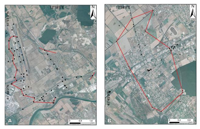
FIGURE II. Contour reconstruction of the peat layer in the two analyzed areas with the boreholes information; A) Maccarese, B) Ostia.
