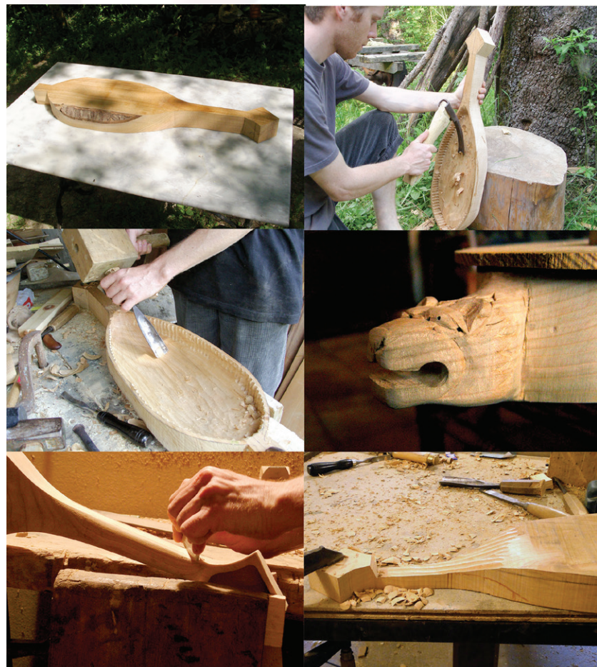
Fig. 29 The body of the instrument is cut out, hollowed out with an adze, finished with a gouge, carved and smoothed out with a scraper (picture: O. Feraud).
