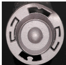
Figure 2: Example of incomplete casting
