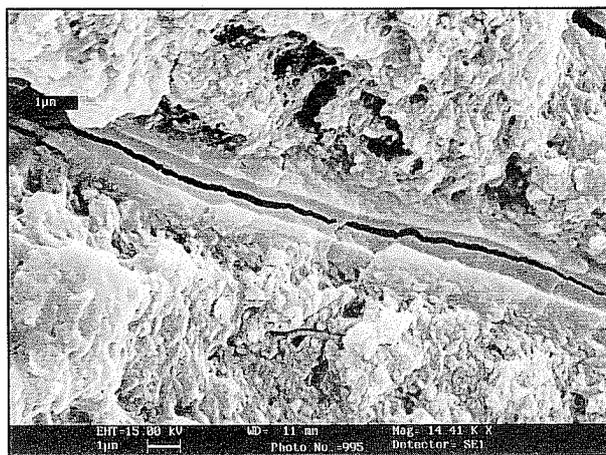
**Fig. 6.** Compound treated with Prompt. The resinous plugs is adhered to the surface of the tubule, but shows a linear fracture along its axis.
