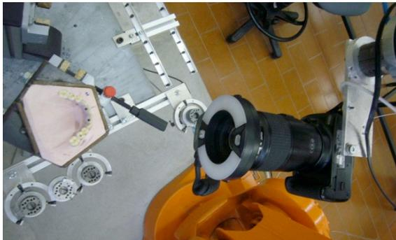
Figure 2 – Left) Schematic representation of the setup to take the photos; the camera was placed in 6 different positions. Right) real view of the setup.
