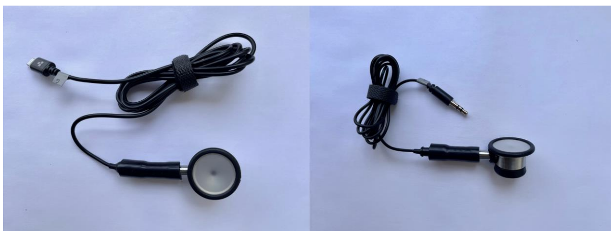
Fig. 2. WDS comprised of a stethoscope head and a short piece of stethoscope tubing which connects the stethoscope head and a lavalier microphone inserted at either side of the tube. 3.5mm TRS audio jack connection (right); lightning connector (left).
