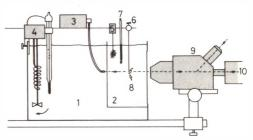
FIGURE 1. Diagrammatic description of the observation chamber for heart rate estimations. 1: Thermostatic bath. 2: Observation aquarium. 3: Light source (light fibre). 4: Heater-cooler with thermostat and homogenizer. 5: Turbulence generator. 6: Manipulator for positioning the organisms. 7: Thermometer. 8: Tethered organism. 9: Stereo microscope. 10: Video camera.
