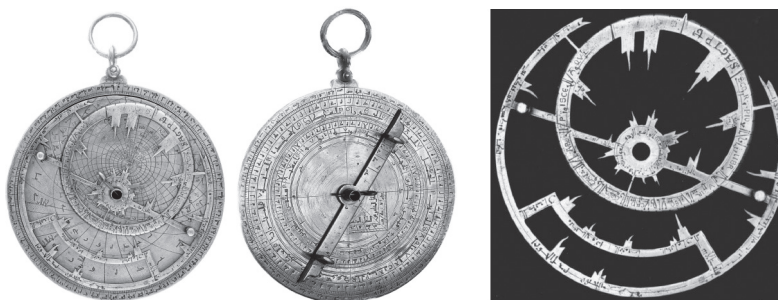
FIGURE 7.5d: The hitherto earliest known Andalusī astrolabe, with an Abbasid-type rete (bearing later Italian inscriptions), astronomical markings featuring several localities (including Medinaceli), and a single shadow square and non-concentric solar scale (cf. Nas̄tūlus’ horary instrument, §5.2) on the back. Images courtesy the British Museum, London.
