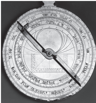
FIGURE 4.2c: A double universal horary quadrant as was standard on the backs of Islamic and European astrolabes. The device has been somewhat misunderstood in the modern literature. Its function is simply to provide a quick means of obtaining a rough estimate of the time of day for any latitude, whereas the astrolabe should give a reasonably accurate value for the latitudes represented by the plates, though more laboriously. It was not generally known that the markings of the universal horary quadrant were based on the standard approximate formula. This is the back of the «astrolabe of Berselius», a 14th-century Picard piece with all numbers in monastic ciphers. Image courtesy of Christie's of London.
