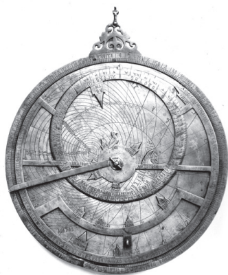
FIGURE 7.5a: The front of the Byzantine astrolabe of 1062. This instrument shows not one iota of external Islamic influence! Image courtesy of the Santa Giulia Museo della Città in Brescia.
