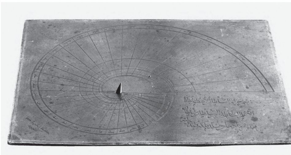
FIGURES 1.1a-c: The front of the universal sundial, the dedication in the lower right of the spiral horary markings. All images courtesy of the owner.
