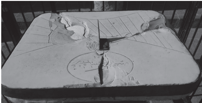
FIGURE 7.3b: One of several images of the Diyarbekir sundial on the internet. It is encased in a metal band, and the column is surrounded by a tall metal railing. The railing and the metal band and also the gnomon have been painted bright blue. Image from https://www.mucadelgazetesi.com.tr/gunes-saati-850-yildir-zamani-gosteriyor .
